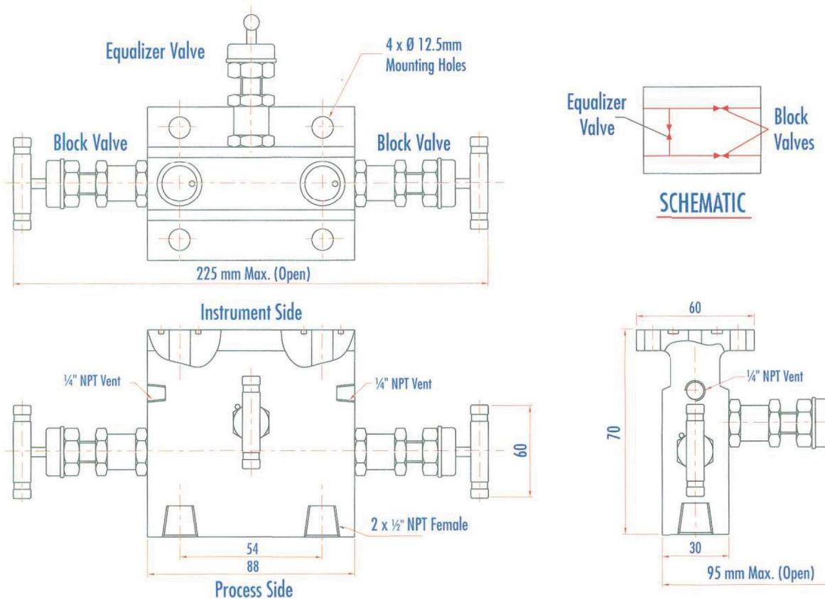
**Model 3WM341** - Stainless steel body, Flange to Flange (Dual Flange type)
