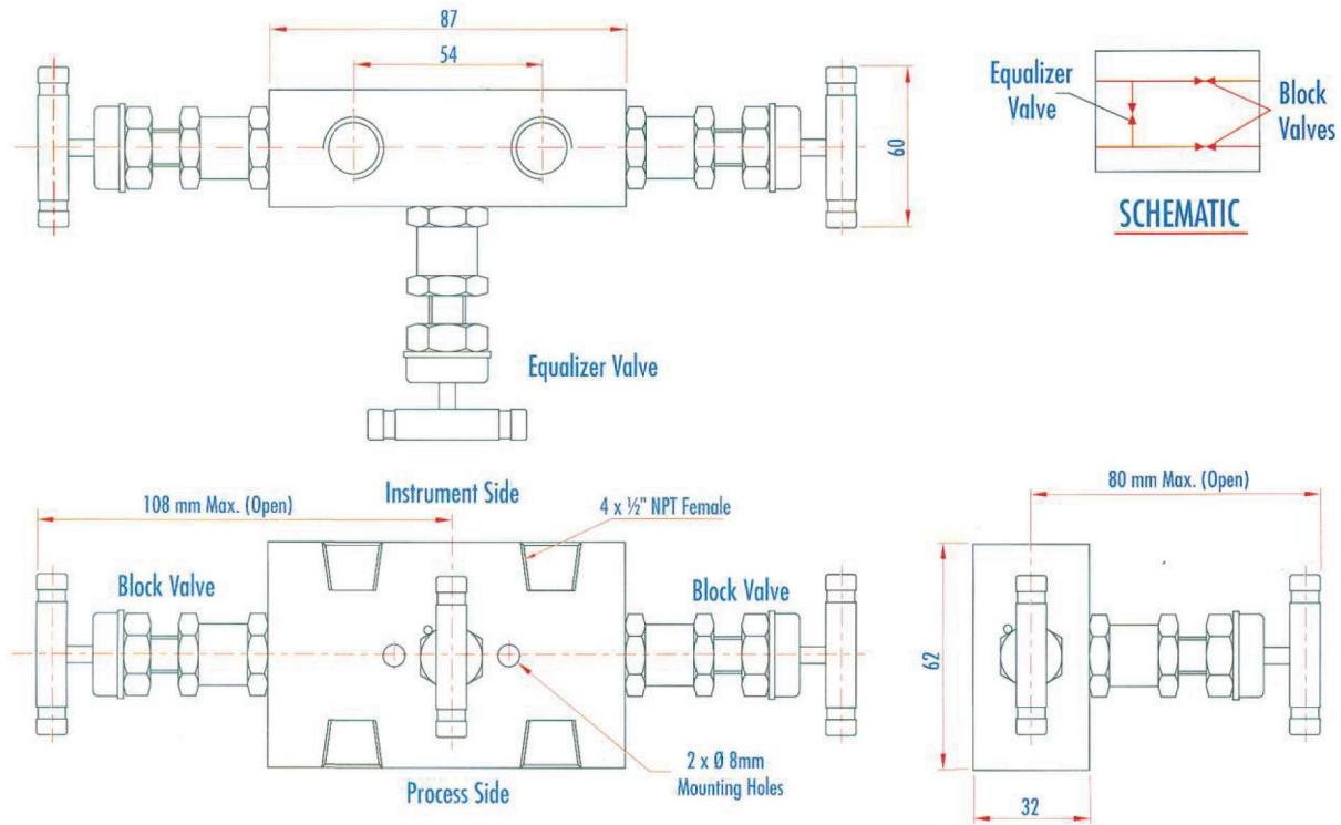
**Model 3WM321** - Stainless steel body, Pipe to Flange (Direct mount type)
